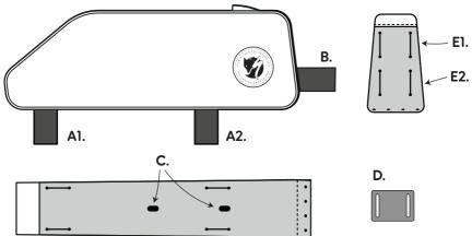
Attach lower two velcro loops (A) towards top tube and front velcro with velcro protective tape (B) towards headset. \* If velcro straps are to long, trim to adapt.
